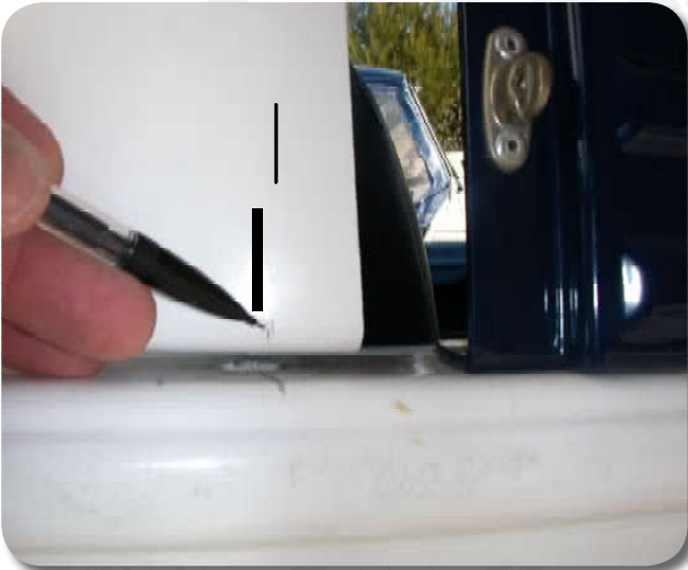
5/ For an easy marking and drilling of the elements, put a mark onto the hole axes on the vehicle.
