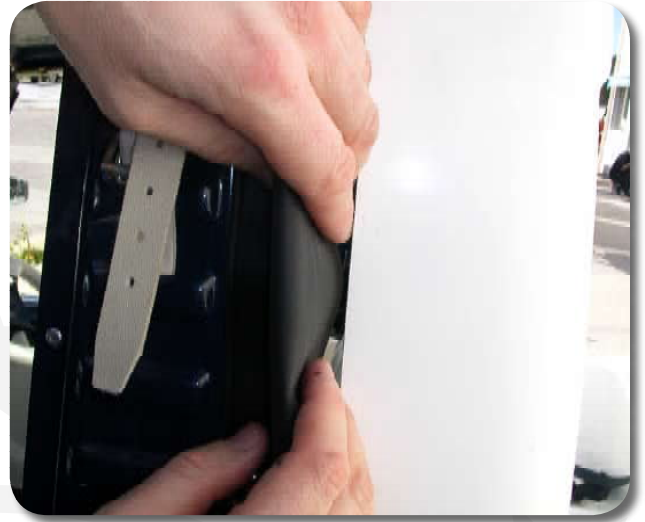
12/ Insert the sleeve inside.
