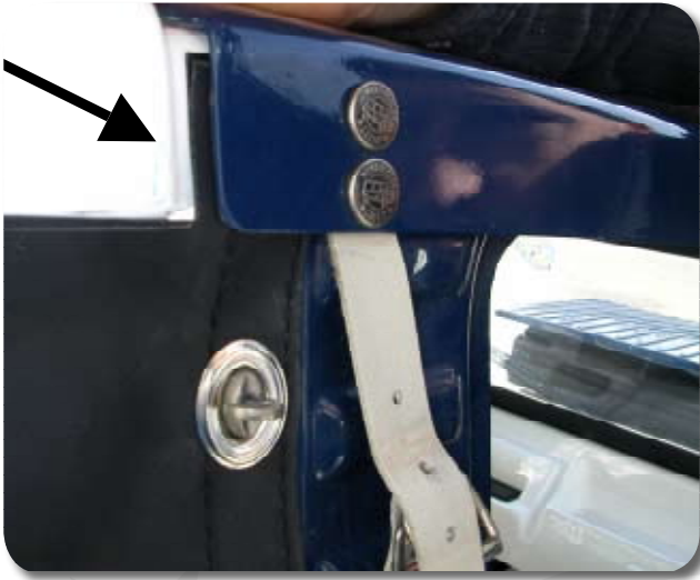
11/ Intercalate the upper part of the sleeve between the roof and the element.
