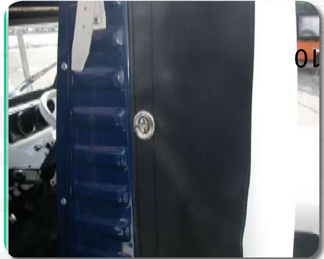
10/ Fix the sealing sleeve with the swivels.
