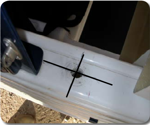
5/ For an easy marking and drilling of the elements, put a mark onto the hole axes on the vehicle.
